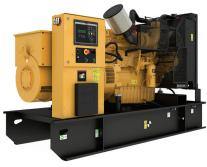
Engine ModelCat® C9 In-line 6, 4-cycle DieselBore x Stroke112mm x 149mm (4.4in x 5.9in)Displacement8.8 L (538 in³)Compression Ratio16.1:1AspirationTurbocharged Air-to-Air AftercooledFuel Injection SystemHEUIGovernorElectronic ADEM™ A4 - G3 Class\* capable
