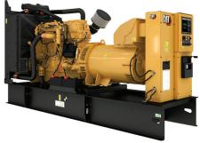
Engine ModelCat® C15 In-line 6, 4-cycle DieselBore x Stroke137mm x 171mm (5.4in x 6.8in)Displacement15.2 L (928 in³)Compression Ratio16.1:1AspirationTurbocharged Air-to-Air AftercooledFuel Injection SystemMEUIGovernorElectronic ADEM™ A4 - G3 Class\* capable
