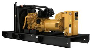
Engine ModelCat® C18 In-line 6, 4-cycle DieselBore x Stroke145mm x 183mm (5.7in x 7.2in)Displacement18.13 L (1106.3 in³)Compression Ratio14:1AspirationTurbocharged Air-to-Air AftercooledFuel Injection SystemElectronic Unit InjectionGovernorElectronic ADEM™ A4 - G3 Class\* capable
