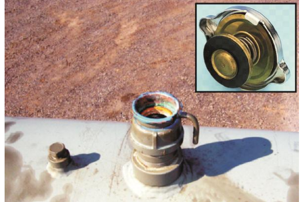
Figure 43: Expansion tank with automotive-type adapter and pressure cap.
