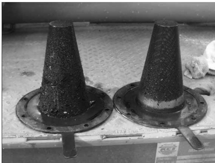
Figure 5.1 – Cooling System Cleaning Screens
