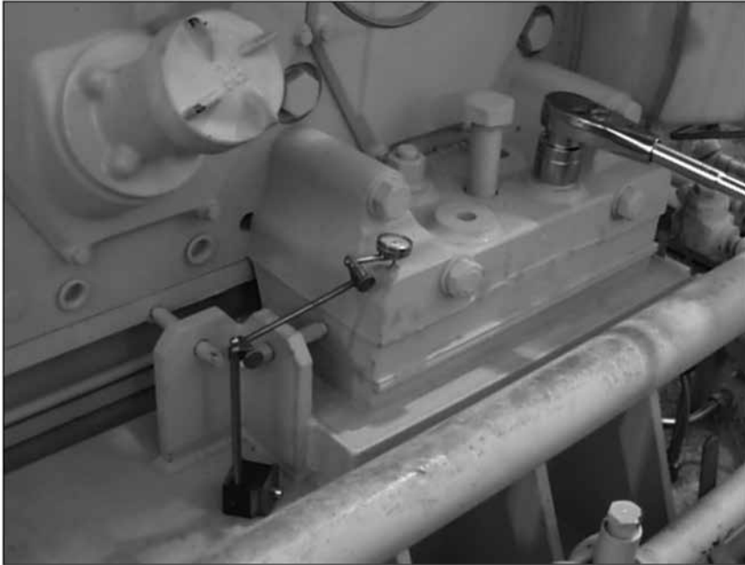
Figure 4.5 – Checking Soft Foot by Loosening Mounting Bolts and Measuring Foot Movement
