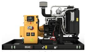
Engine Model 3.6L TCAC Inline No. of Cylinders 4 Bore x Stroke 105.54 mm x 102.9 mm 3.6 Liter Displacement 9.7:1 **Compression Ratio** Turbocharged & Aftercooled Aspiration Fuel / Ignition System Electronic Regulator / Spark Ignition Governor Electronic - G2 Class\* capable
